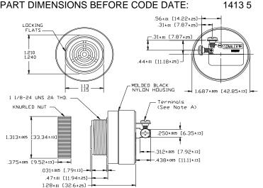
NOTE A: TERMINALS-.032 BRASS TIN PLATED, TAPPED FOR #6-32 SCREW. TVD #6-32 NICKEL PLATED BRASS SCREWS INCLUBED. WILL ACCEPT 1/4\* QUICK CONNECT.
