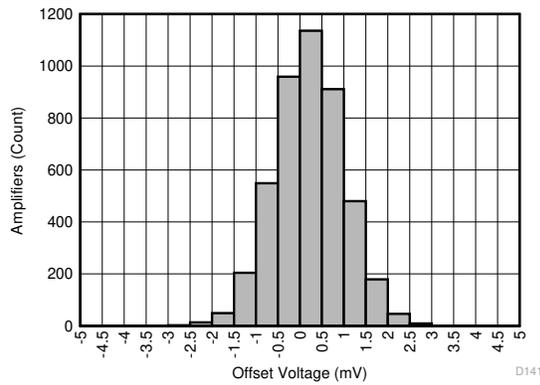
$\mu = -0.28\text{ mV}$        $\sigma = 0.8\text{ mV}$       4555 units tested
