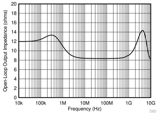
**Figure 8-7. Open-Loop Output Impedance ( $Z_{OL}$ ) vs Frequency**
