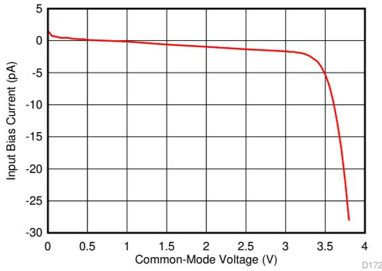
Figure 6-39. Input Bias Current vs Input Common-Mode Voltage
