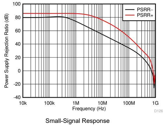
Figure 6-26. Power Supply Rejection Ratio vs Frequency
