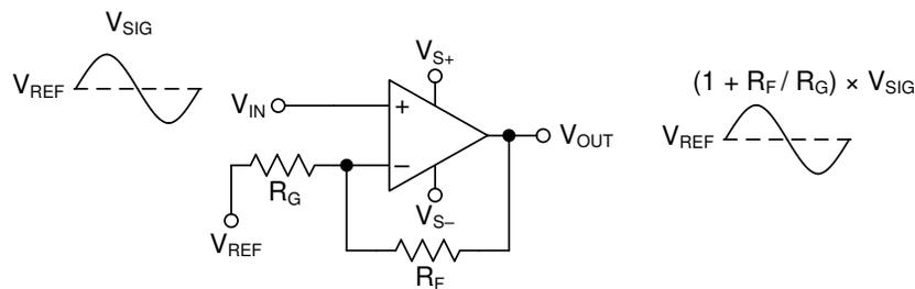
**Figure 8-1. Noninverting Amplifier**
