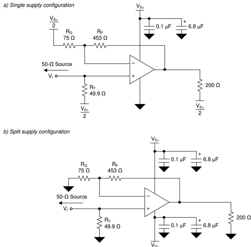
Figure 10-1. Split and Single Supply Circuit Configuration
