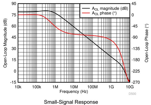
Figure 6-10. Open-Loop Magnitude and Phase vs Frequency
