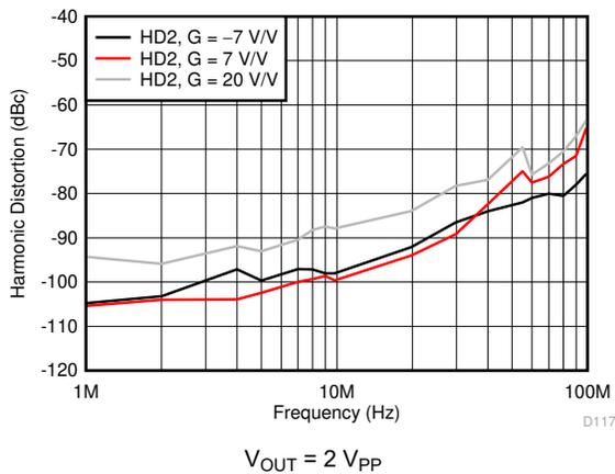
Figure 6-17. Harmonic Distortion (HD2) vs Gain
