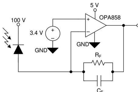
**Figure 9-1. Transimpedance Amplifier Circuit**
