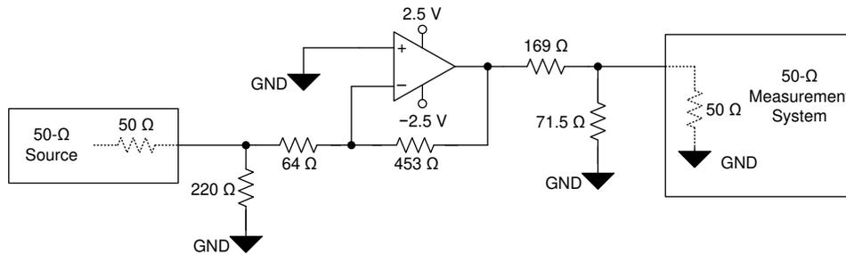
**Figure 7-2. Inverting Configuration (Gain =  $-7$  V/V)**
