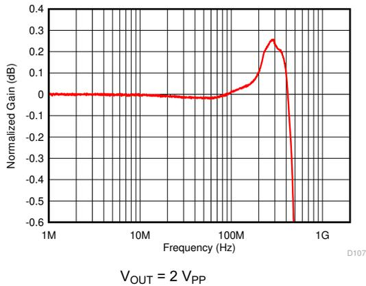
Figure 6-7. Large-Signal Response for 0.1-dB Gain Flatness
