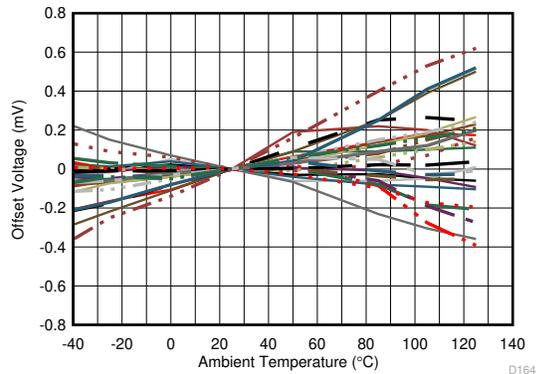
$\mu = 1\ \mu\text{V}/^\circ\text{C}$        $\sigma = 2.2\ \mu\text{V}/^\circ\text{C}$       28 Units Tested
