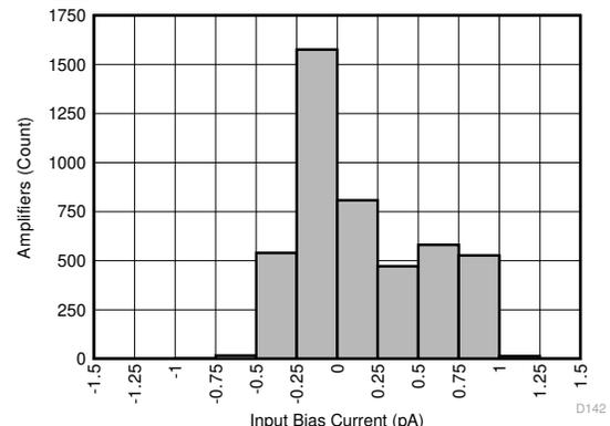
$\mu = -0.1\text{ pA}$        $\sigma = 0.39\text{ pA}$       4555 units tested
