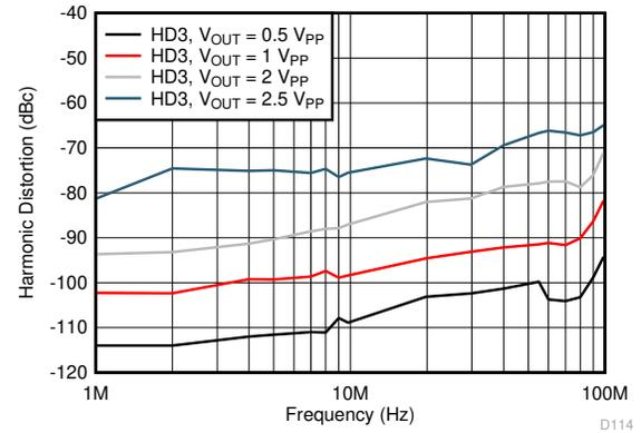
Figure 6-14. Harmonic Distortion (HD3) vs Output Swing
