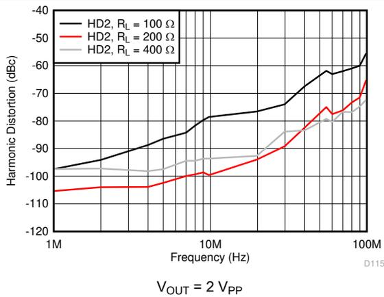
Figure 6-15. Harmonic Distortion (HD2) vs Output Load
