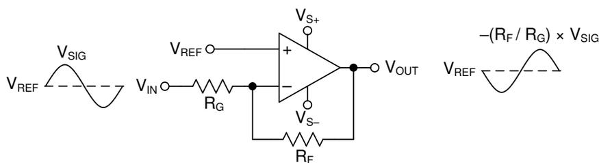
**Figure 8-2. Inverting Amplifier**
