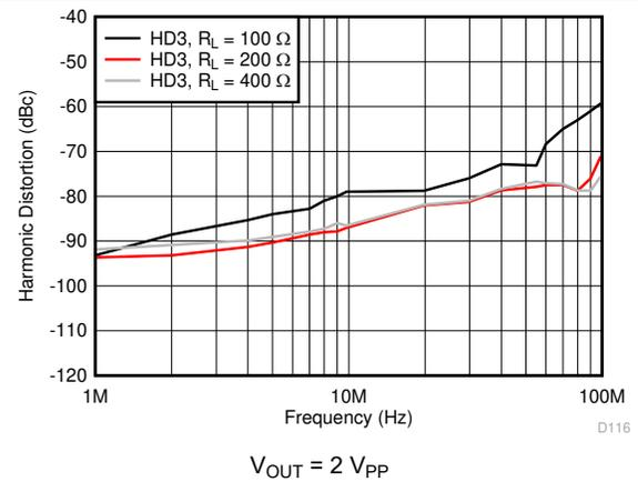
Figure 6-16. Harmonic Distortion (HD3) vs Output Load
