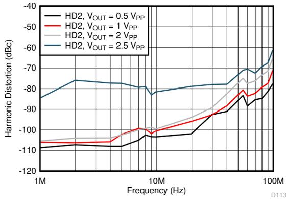
Figure 6-13. Harmonic Distortion (HD2) vs Output Swing
