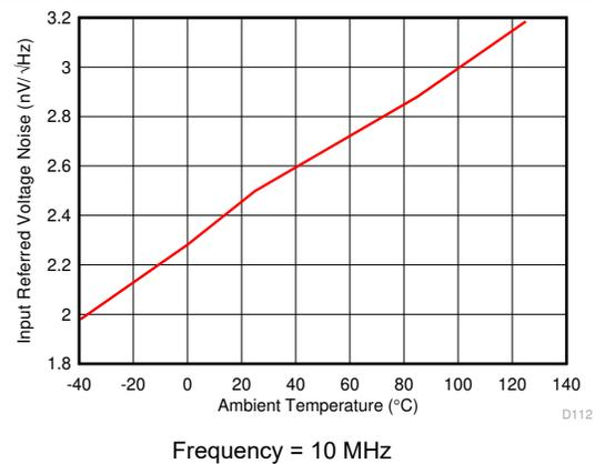
Figure 6-12. Voltage Noise Density vs Ambient Temperature
