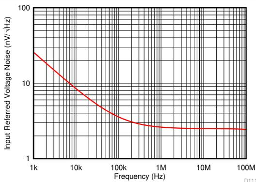
Figure 6-11. Voltage Noise Density vs Frequency
