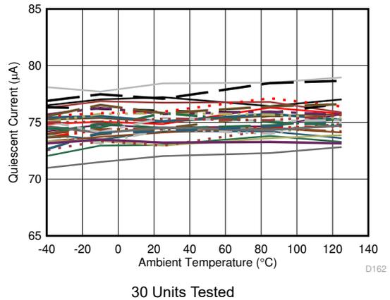
Figure 6-29. Quiescent Current (Amplifier Disabled) vs Ambient Temperature
