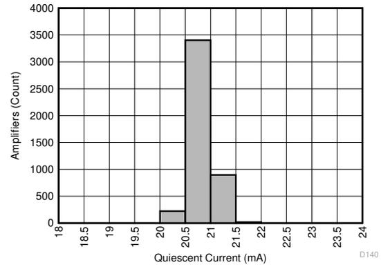
$\mu = 20.35\text{ mA}$        $\sigma = 0.2\text{ mA}$       4555 units tested
