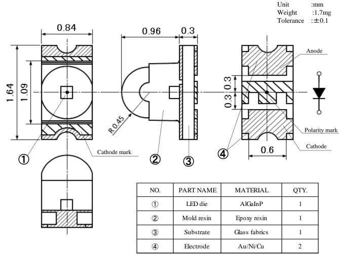
Note: The cutting burr of the substrate and electrodes doesn't contain size of the product.
