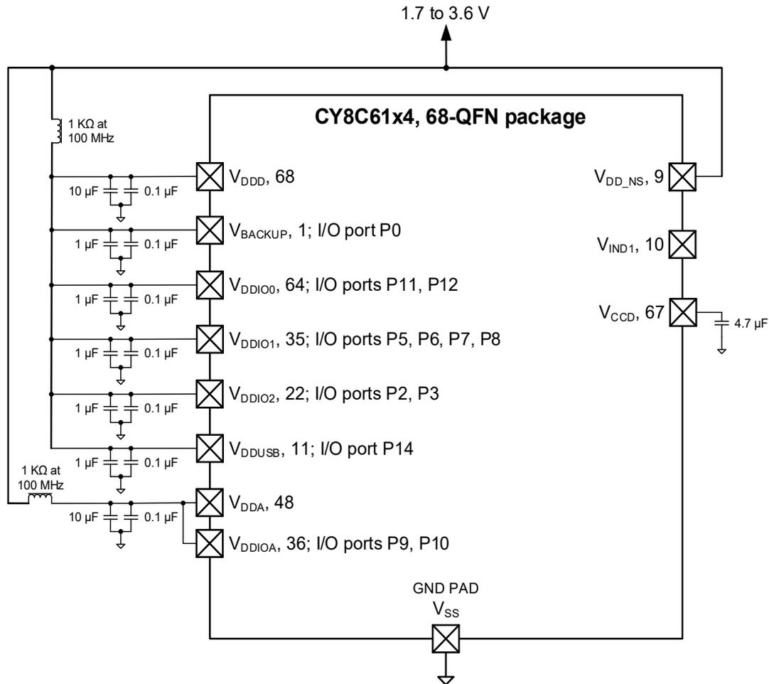
There are as many as eight  $V_{DDx}$  supply pins, depending on the package, and multiple  $V_{SS}$  ground pins. The power pins are:
