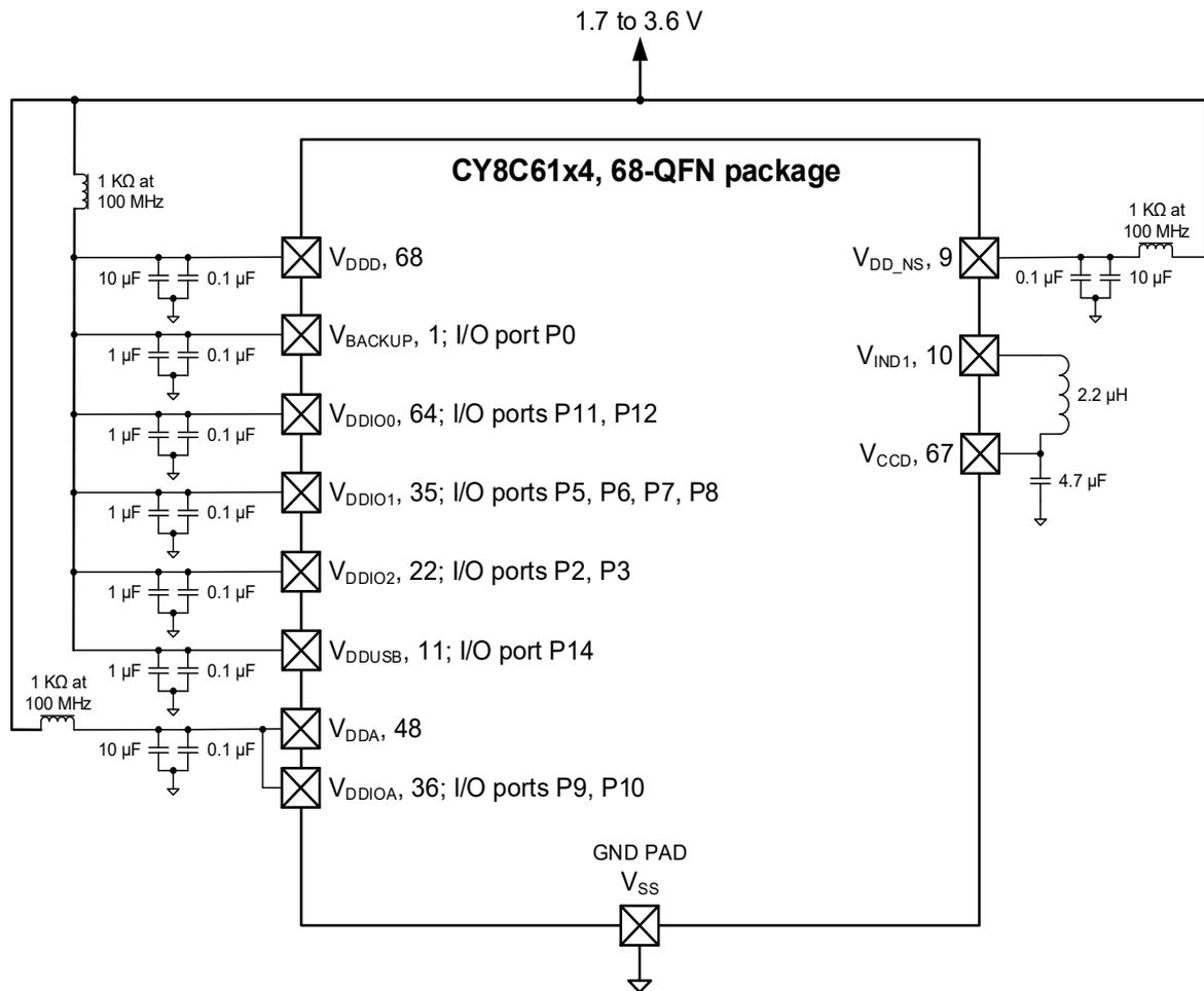
**Figure 15. 68-QFN (No Buck) Power Connection Diagram**
