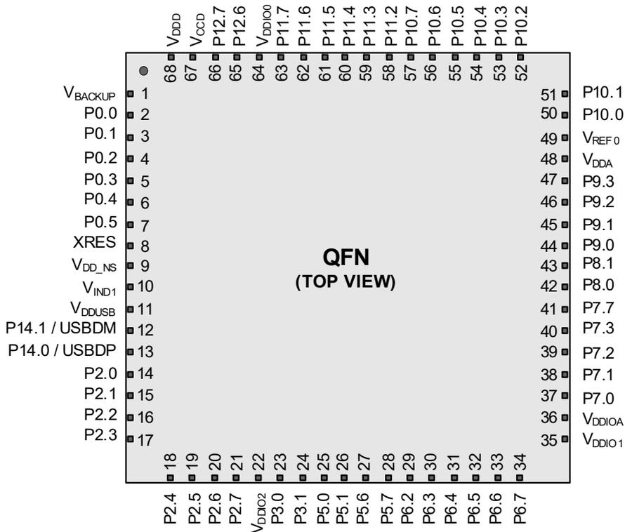
Each port pin has multiple alternate functions. These are defined in Table 7. The columns ACT #x and DS #y denote active (System LP/ULP) and Deep Sleep mode signals respectively.
