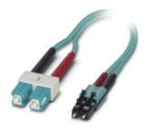
Assembled FO cable, zip cord cable, multi-mode fiberglass 50/125  $\mu$ m, OM3, plug: LC/SC duplex, degree of protection: IP20, for installation in cable ducts or control cabinets, length: 2 m
