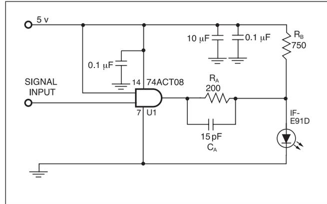
FIGURE 3. Test application circuit ( $I_f = 22\text{mA}$ ).
