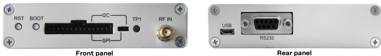
Figure 2: EVK-M8U evaluation unit – front and rear panels
