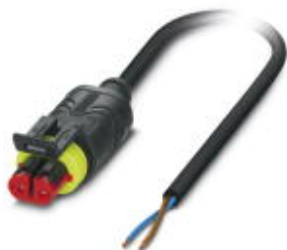
Sensor/actuator cable, 2-position, PUR halogen-free, black-gray RAL 7021, free cable end, on Socket straight Superseal Clip locking, cable length: 1.5 m
