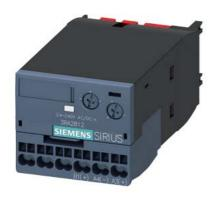
electronic timing relay, off delayed, with control signal and semiconductor output, time range 0.05-100 s, 24-240 V AC/DC, 50/60 Hz, varistor for attenuation of the contactor coils integrated, spring-loaded terminal, can be snapped onto the front on contactors 3RT201 / 3RT202 and auxiliary contactors 3RH2
