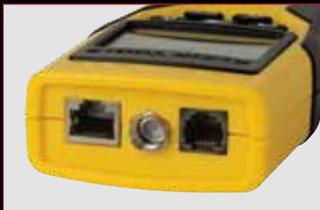
RJ45, F-Connector and RJ11/12 Jacks
