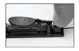
Grasp the left fiber about 2 inches from the holder and push the fiber in until it bows about 1/8 to 1/4 inch (3mm to 6mm). Push down on the actuation lever until the Fibrlok II Splice is actuated. An audible click can be heard and you should feel the splice cap snap down into place when completely closed. The cap should be level with the Fibrlok splice top surface.
