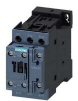
power contactor, AC-3 12 A, 5.5 kW / 400 V 1 NO + 1 NC, 24 V DC 3-pole, Size S0 screw terminal upright mounting position
