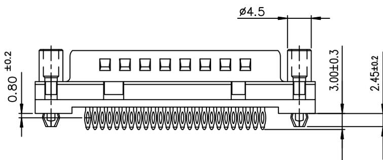
PC board drilling dimensions(after plating)
