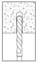
Using the proper drill bit size, drill a hole into the base material to the required depth.
