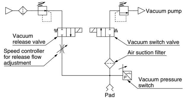
If a filter is required on the release pressure side, a different filter should be prepared.
