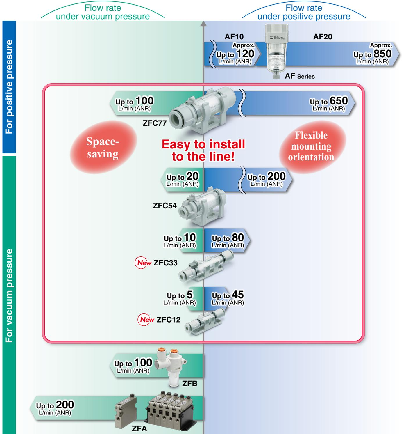
Flow rate (positive pressure) conditions: Supply pressure of 0.7 MPa, Pressure drop of 30 kPa
