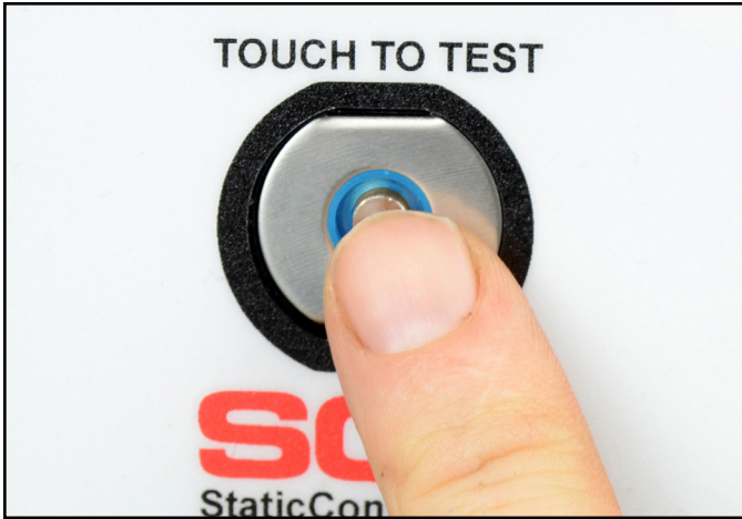
Figure 11. Bridging the test switch's contacts to initiate the test
