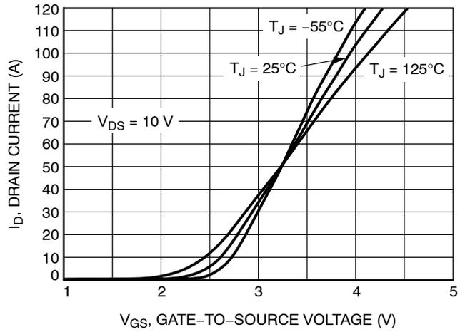
Figure 2. Transfer Characteristics
