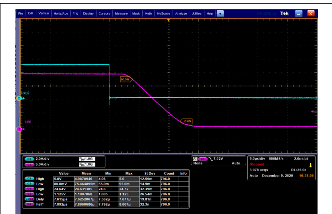
Figure 10-3. Recessive to Dominant Propagation
