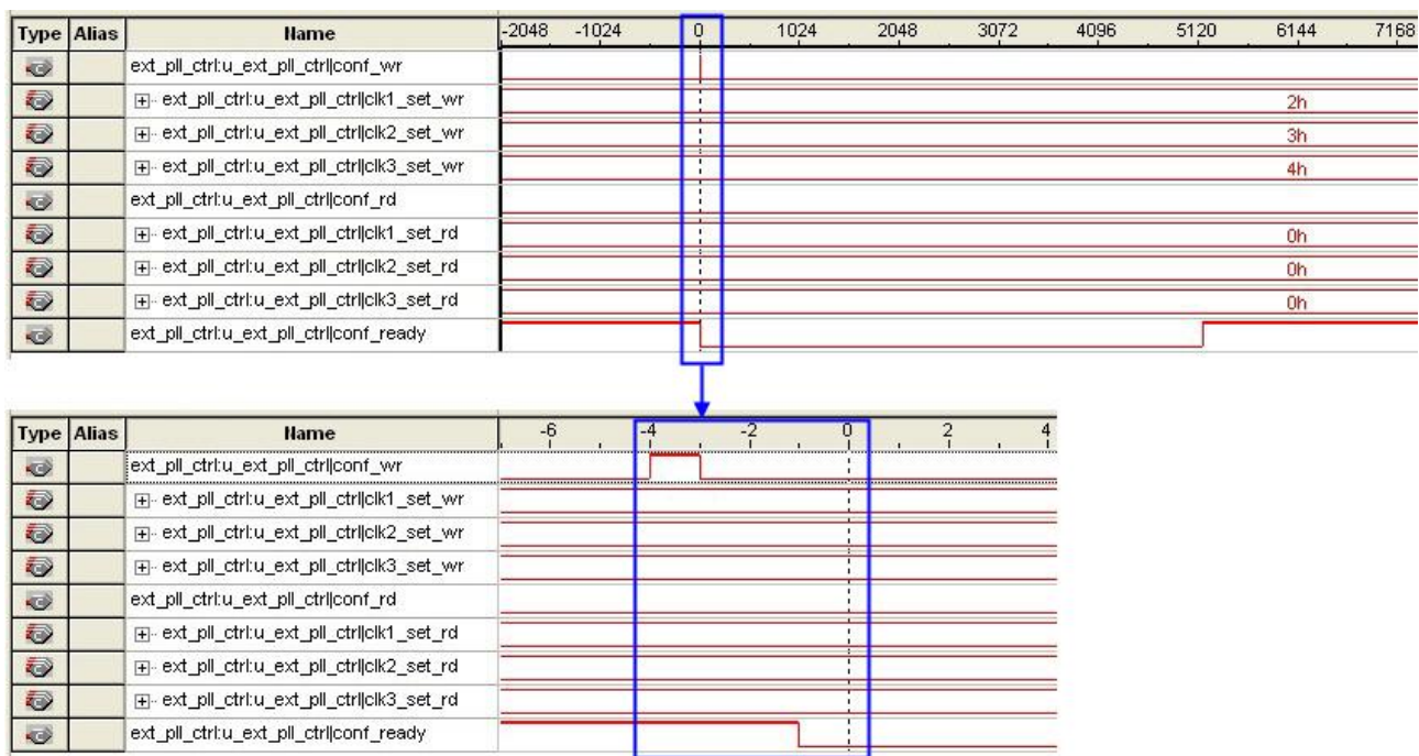
Figure 5-4 Write Timing Waveform
