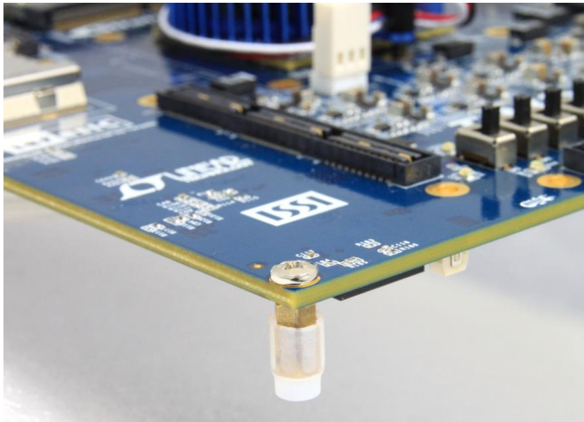
Figure 1-4 Mount Silicon Foot Stands
