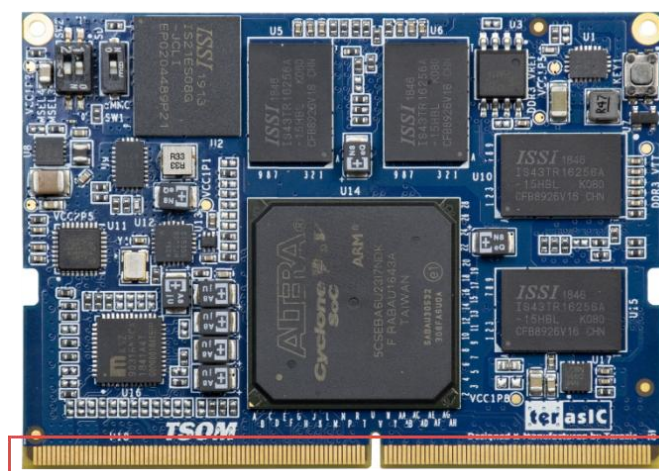
Figure 3-12 260-pin edge connector on the TSoM module
