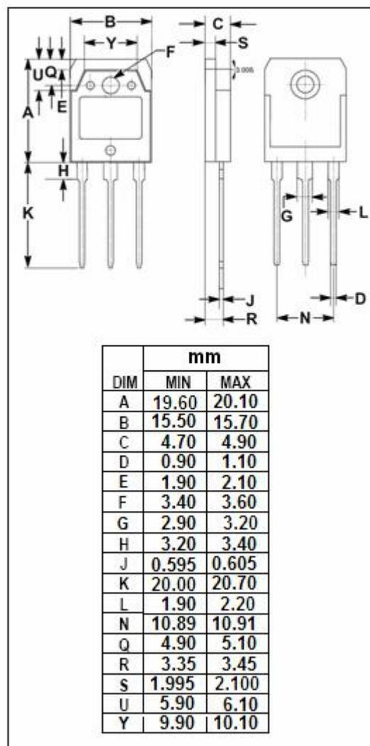
**isc Silicon NPN Power Transistor**
