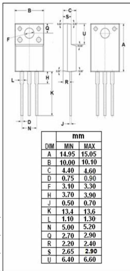
**isc N-Channel MOSFET Transistor****AOTF2618L****ELECTRICAL CHARACTERISTICS**T<sub>C</sub>=25°C unless otherwise specified
