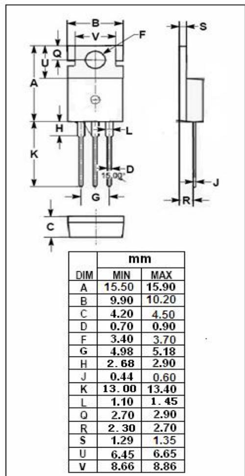
**isc N-Channel MOSFET Transistor****IPP023N04N,IIPP023N04N****ELECTRICAL CHARACTERISTICS****T<sub>c</sub>=25°C unless otherwise specified**
