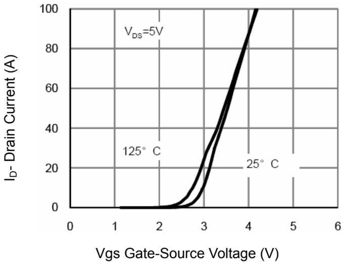
**Figure 2 Transfer Characteristics**
