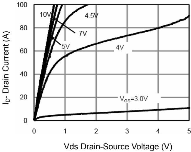
**Figure 1 Output Characteristics**
