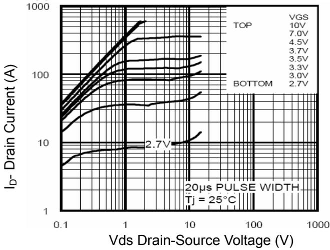
**Figure 1 Output Characteristics**
