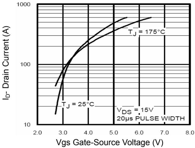
**Figure 2 Transfer Characteristics**
