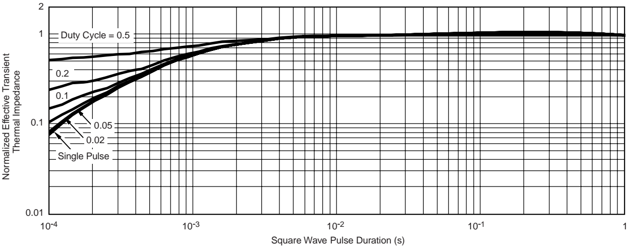
Normalized Thermal Transient Impedance, Junction-to-Case
